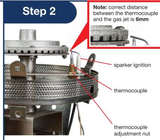
Undo the thermocouple adjustment nut and lower the thermocouple as shown above. Tighten the adjusment nut. Replace the lantern mesh and secure with screws.
